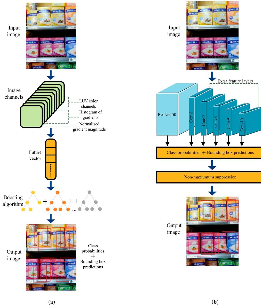
Figure 4. (a) The steps of the ACF in Stage-1. (b) The steps of the SSD in Stage-1. (Red frames indicate the obtained bounding boxes predictions.)
