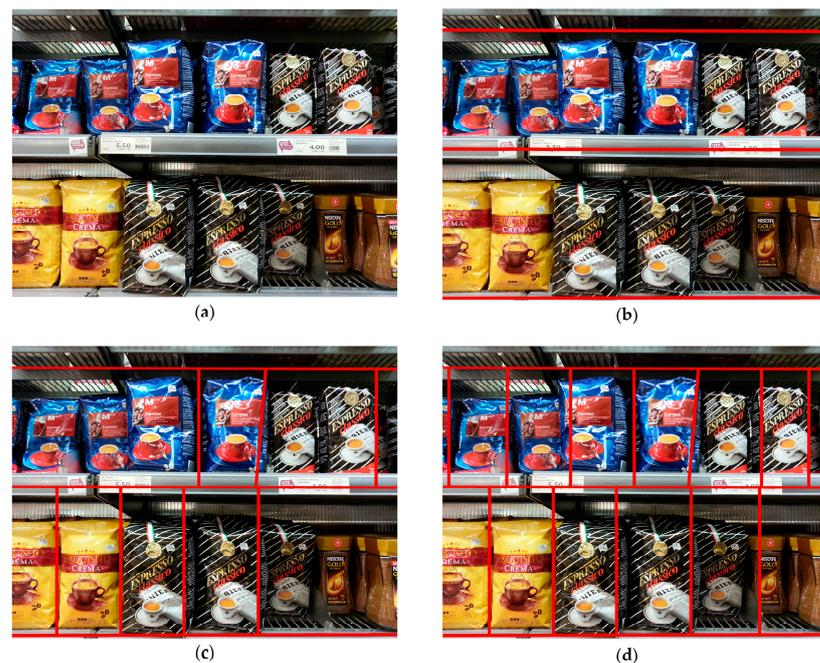
**Figure 3.** The steps of the proposed traditional computer vision approach in Stage-1: (a) original shelf image; (b) shelf image with detected shelf lines after first step; (c) shelf image with detected product regions after second step; (d) shelf image with completed product regions after third step.
