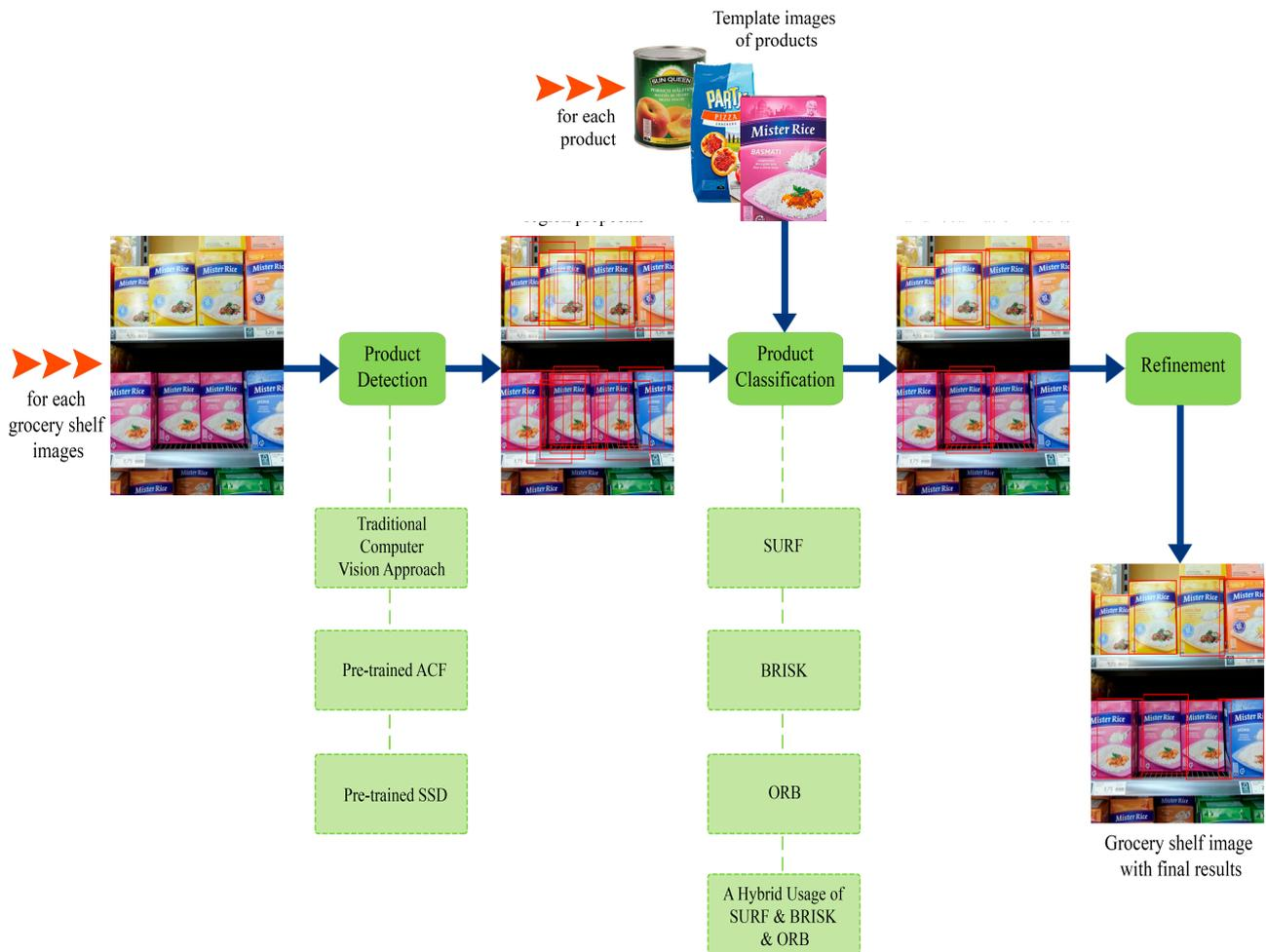
**Figure 2.** Multi-stage end-to-end recognition process. (Red frames indicate the bounding boxes obtained from each step.)
