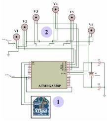
Fig. 3 Robot hand unit connections. (1) rf module, (2) servo motors
