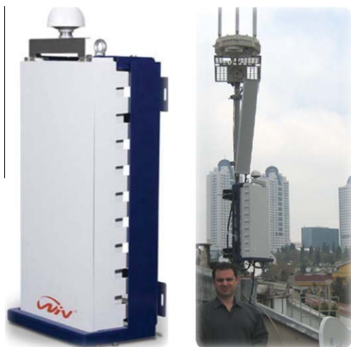
Fig. 2.8. WiNetworks WiN7000 series base station and field-mounted version.
