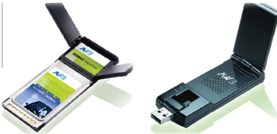
Fig. 2.10. AWB PC200 WiMAX PCMCIA card and US210 WiMAX USB adaptor.
